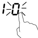
3. Using the "+" or "-" buttons ,you can realize the set the timer from 1 to 99 minutes.
