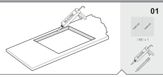
Cut out worktop to the template dimensions with suitable equipment and seal the cut edge with appropriate sealant.
