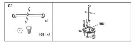
Lift up the burners and unscrew the nozzle using an dedicated tool and replace the nozzles with those designed for LPG gas supply. (see table on page 16)
