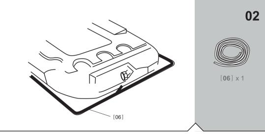
Stretch out the supplied seal along the underside edge of the hob, ensuring the ends overlap.
